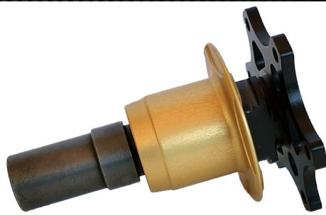
► QUICK RELEASE: **STEERING COLUMN HUB SHAFT**
